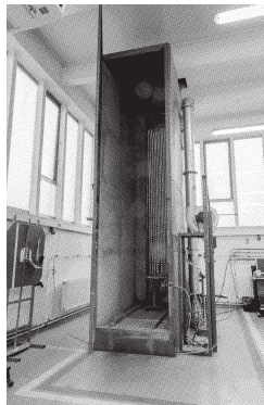
Test of fire propagation in bundles
